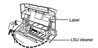
4 Replace the toner cartridge, close the top cover, and turn the printer on.
