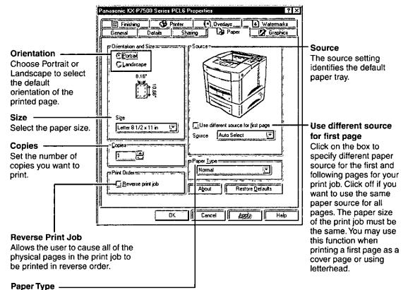
The Paper type setting lets you specify the type of print material installed in each tray.
