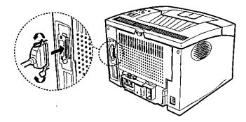
Connect the other end of the parallel interface cable into the appropriate parallel connector on your computer and tighten the screw.
