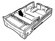
Slide the cassette completely into the printer.
