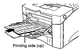
Adjust the paper guide to the size of the paper inserted by pushing the guide.
